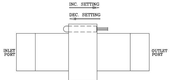
**Caution:** *Do not overtighten the switch holding set screw — this is a cone point screw that digs into the tube with light pressure. (In some cases, it might be necessary to reverse the switch tube end-for-end to locate the new actuation point. This is a normal procedure.)*
