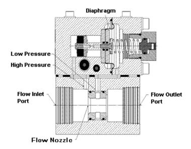
**IMPORTANT:** Because of the magnetic movement, this instrument should <u>never</u> be mounted in direct contact with a steel surface. Otherwise a calibration shift will occur. Mount the instrument so that the pressure body is at least 1" away from ferrous materials.
